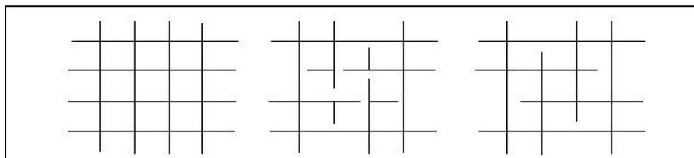
Figure 1. Traffic structures, (from left to right) grid or lattice, organic or tree, mixed or limited access.
