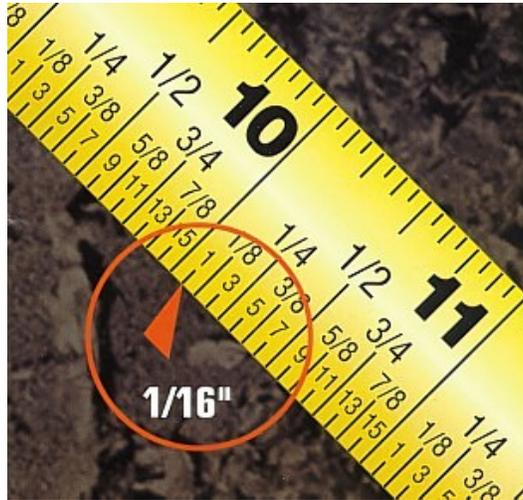
A tape measure blade is marked both in inches and in feet. The end hook always appears to be loose and this is intentional. It's designed to slide a distance equal to its own thickness so both inside and outside measurements will be accurate.
