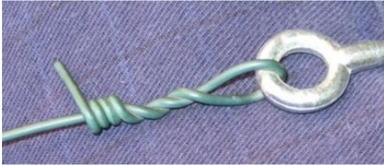
The Haywire Twist and Barrel Roll tie with a clearer background (my sleeve)!
