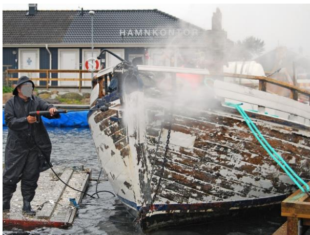
Figure 6-5. Photo: Almost all removed paint from boatyards are spilled to the sea or shore
