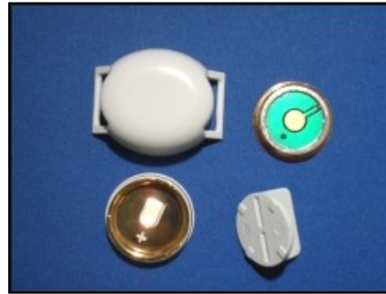
Project Lifesaver wristband shown with its internal transmitter removed for inspection
