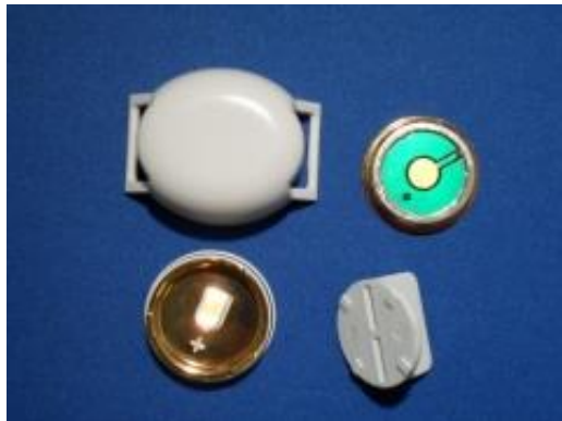
Project Lifesaver wristband shown with its internal transmitter removed for inspection
