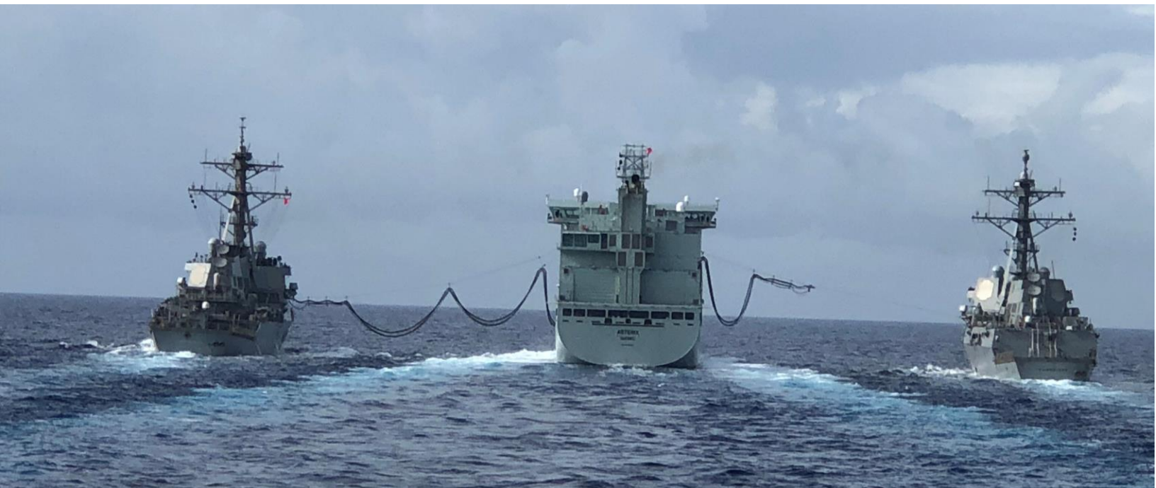
Figure 2: The MV Asterix refuelling accompanying U.S. Navy destroyers during sea trials in the Caribbean. This was the first refuelling of American warships conducted by the Asterix. (Source: Matthew Fisher)
