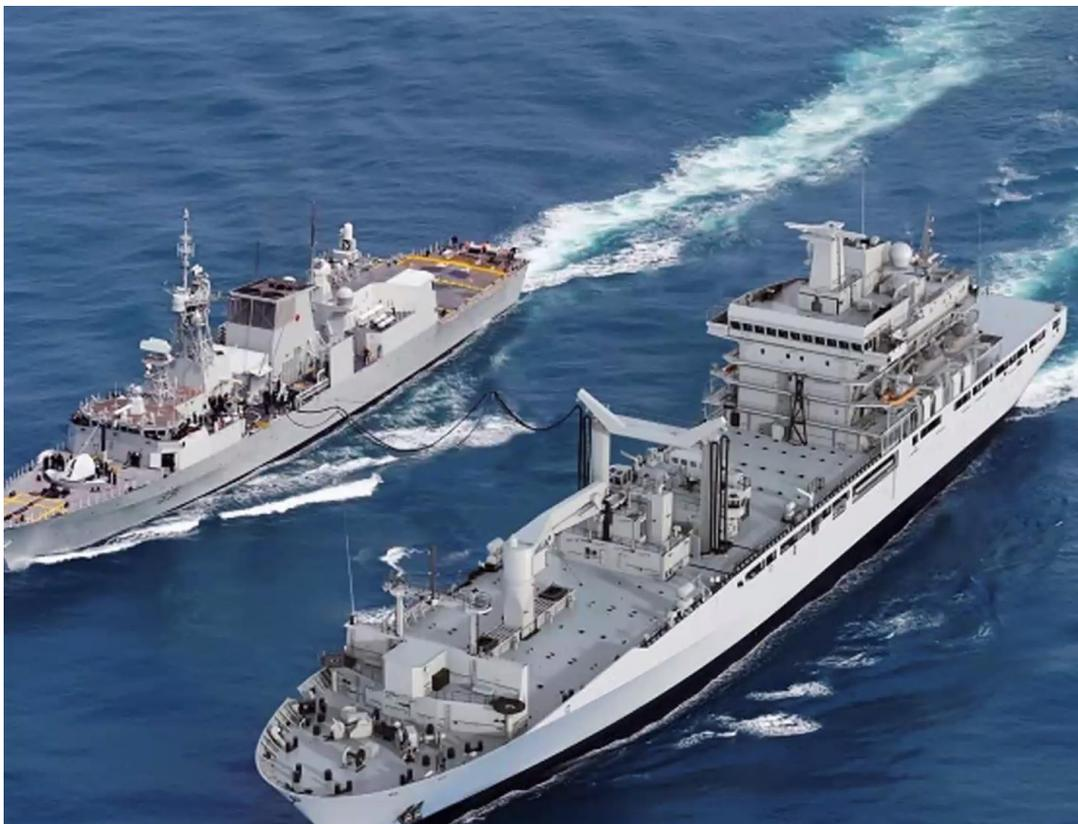
Figure 3: Artist's rendering of the JSS supporting a Halifax-class vessel during replenishment at sea
