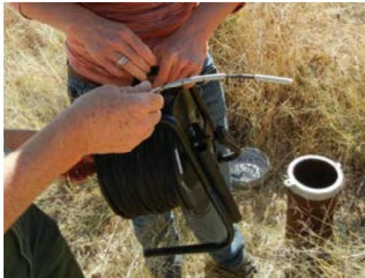
*Routine monitoring is essential to ensuring negative conditions do not impact shallow wells. The device pictured here measures depth to groundwater.*
