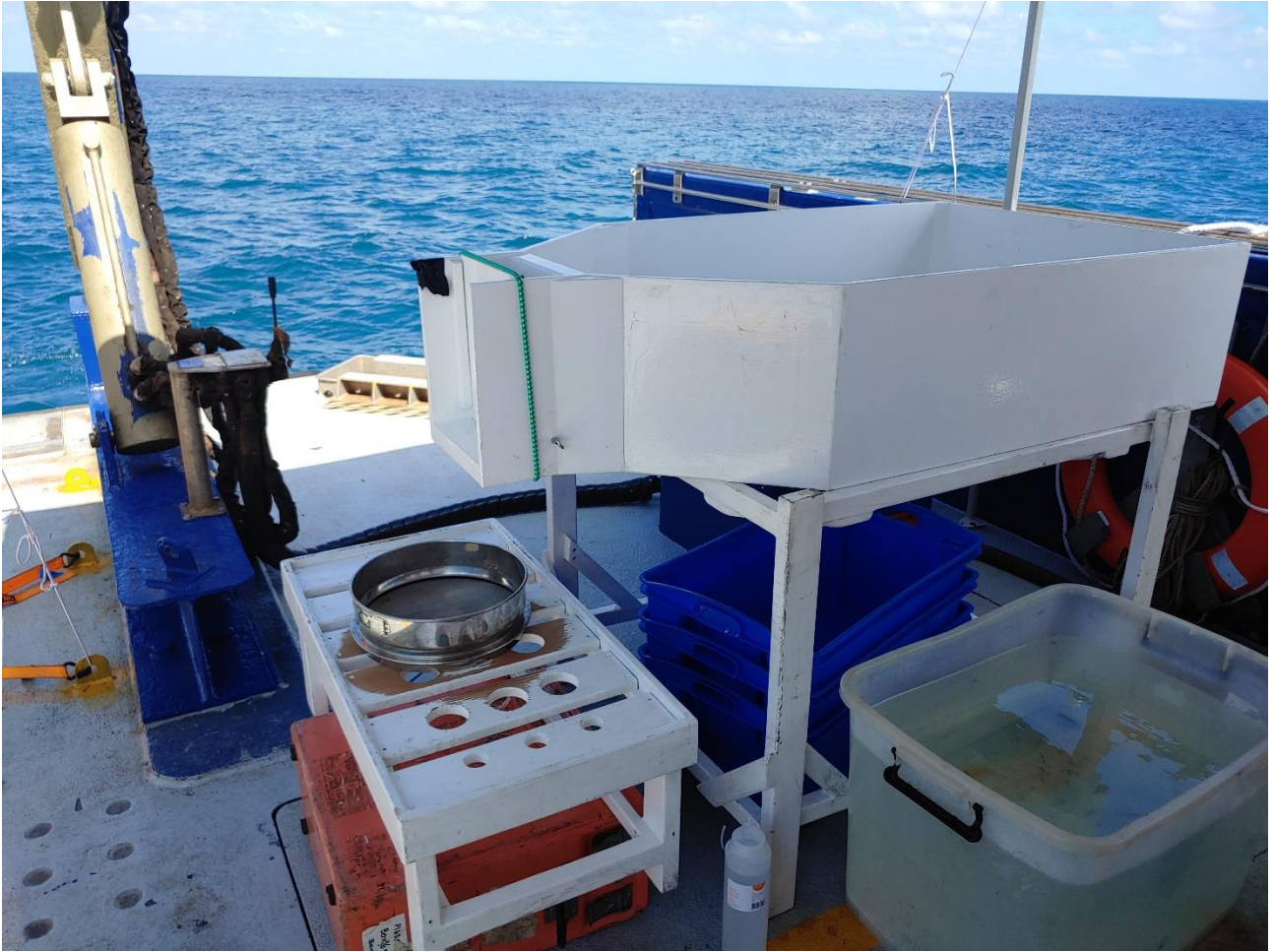
Plate 2-2: Infauna filtering table set up on the Lauri-J
