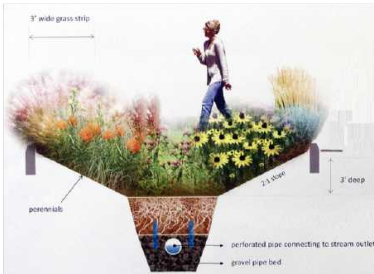
FIGURE 1: EXAMPLE OF A ROADSIDE BIOSWALE
