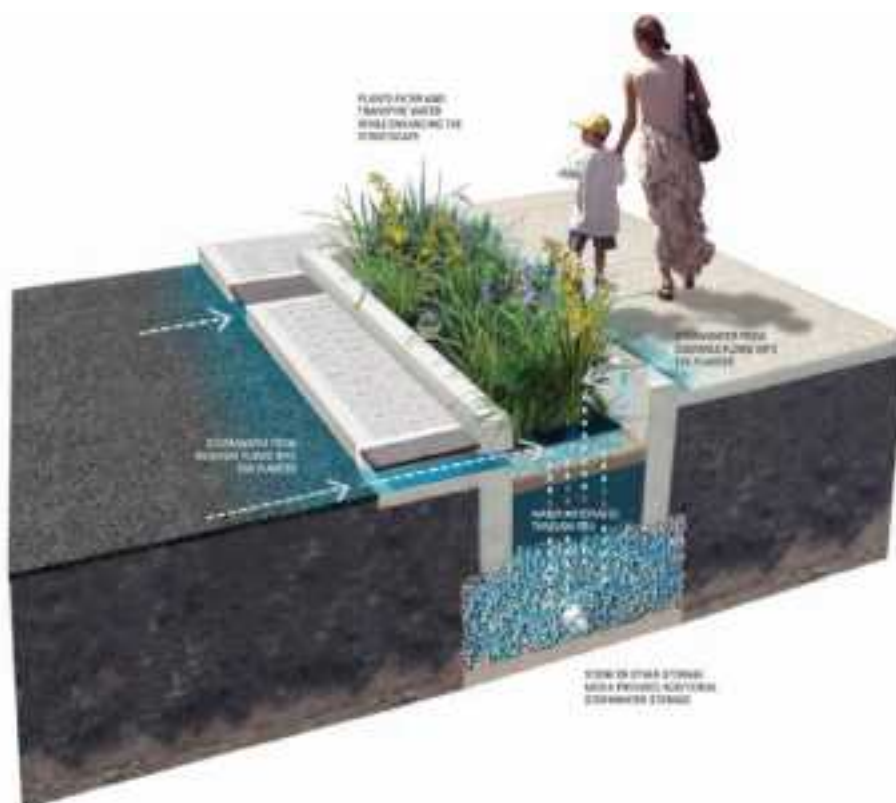
FIGURE 16: VIEW OF A GREEN STREET DESIGN ELEMENT (STORMWATER PLANTER).
