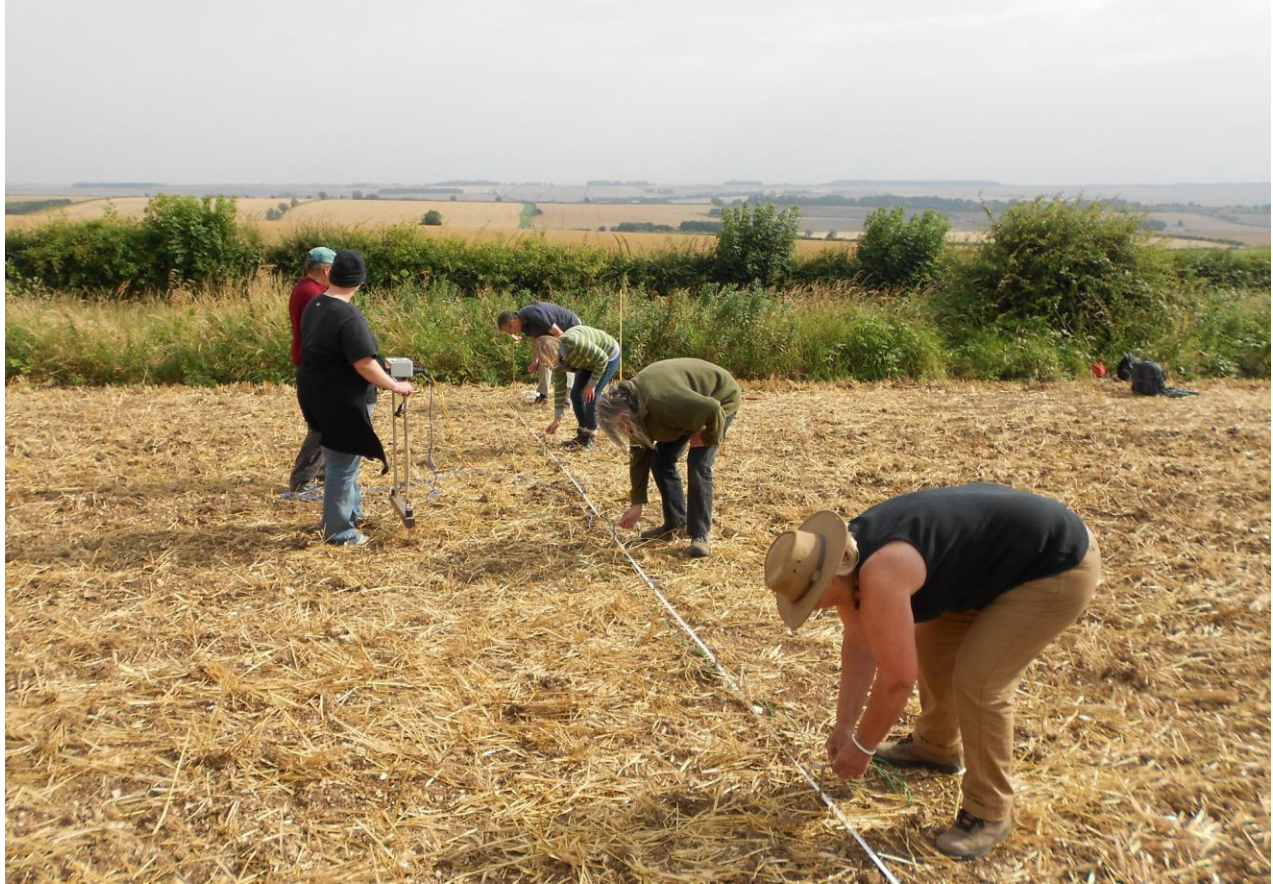
Taking readings for a pseudo-section profile on a LEADER Project site.
