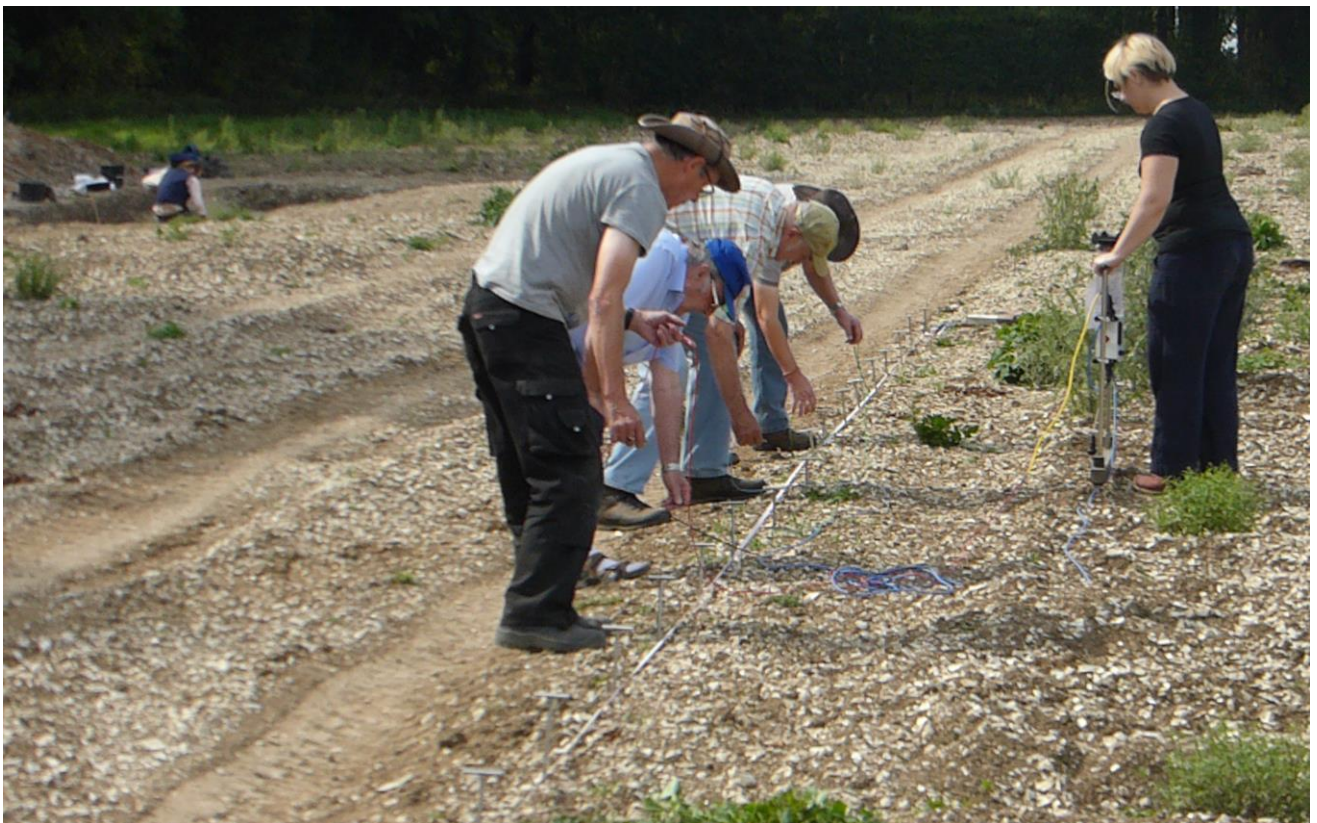
Excavating at Kipling House Farm (top) and using the resistivity meter to take readings for a pseudo section at the site. Photos: Peter Halkon
