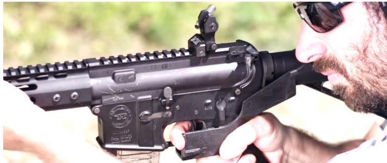
**Photograph Two:** Trigger comes into contact with stationary index finger.
