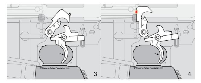
While the empty casing is being ejected from the firearm, the bolt carrier slides rearwards and the hammer is pushed back towards the disconnector. The disconnector grabs and holds the hammer, preventing it from firing another round without the trigger being "reset." Images 5-6. Indeed, unlike with a machinegun, keeping the trigger depressed actually prevents gun from firing again because the disconnector keeps hold of the hammer.
