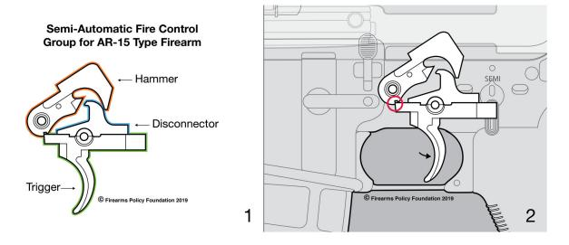
When the firearm is set to fire, the hammer rests on the internal edge of the trigger. Image 2. Causing the trigger to move rearward releases the hammer, which strikes the firing pin and results in a single round being discharged. Images 3-4.
