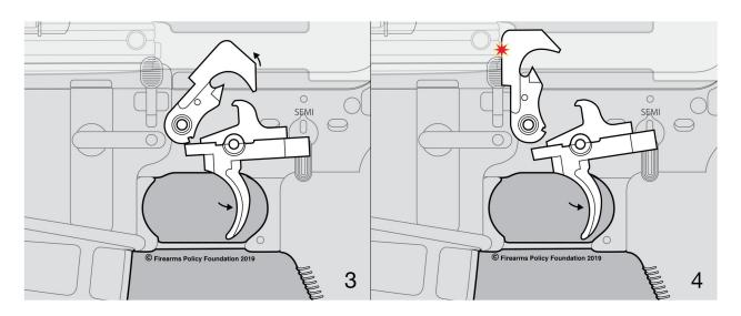
While the empty casing is being ejected from the firearm, the bolt carrier slides rearwards and the hammer is pushed back towards the disconnector. The disconnector grabs and holds the hammer, preventing it from firing another round without the trigger being "reset." Images 5-6. Indeed, unlike with a machinegun, keeping the trigger depressed actually prevents gun from firing again because the disconnector keeps hold of the hammer.
