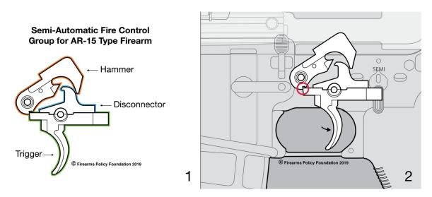
When the firearm is set to fire, the hammer rests on the internal edge of the trigger. Image 2. Causing the trigger to move rearward releases the hammer, which strikes the firing pin and results in a single round being discharged. Images 3-4.
