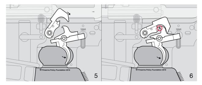
A second function of the trigger occurs when the trigger is released and allowed to move forward, causing the disconnector to let go of the hammer, which then again rests on the
