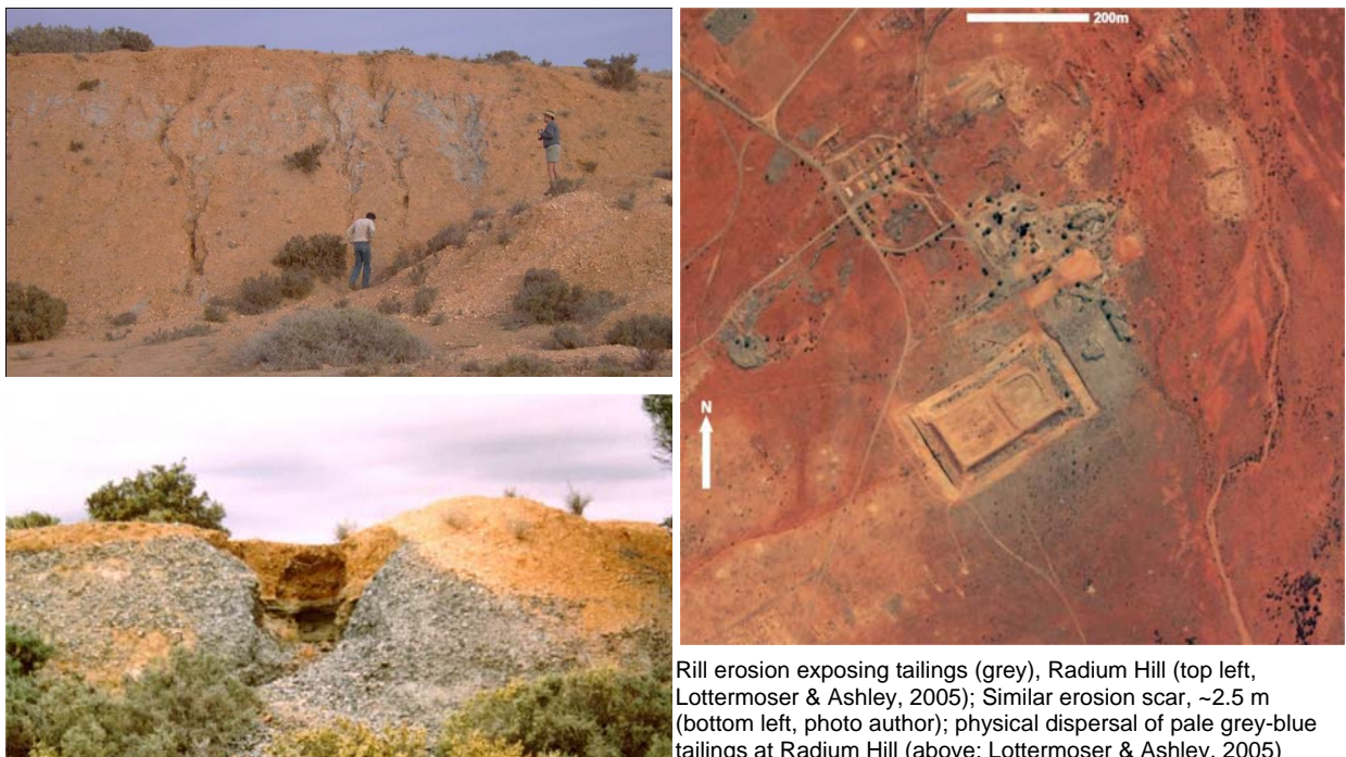
Figure 8: Ongoing erosion problems exposing radioactive tailings at the rehabilitated Radium Hill project, north-eastern South Australia
