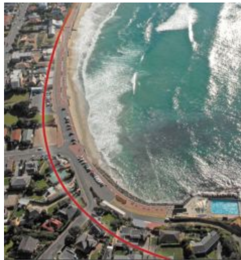
Figure 1: St Clair seawall: red line outlining the beaches equilibrium state.
