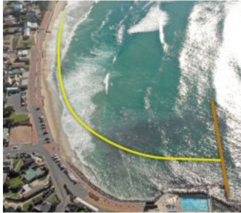
Figure 2: St Clair seawall: yellow lines outlining the implementation of a breakwater instead.
