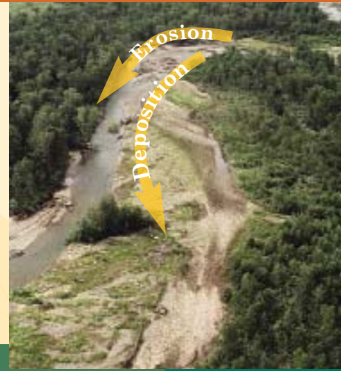
Streams erode the outside of meanders and deposit materials downstream on the inside of meanders. The right vegetation slows the rate of erosion.
