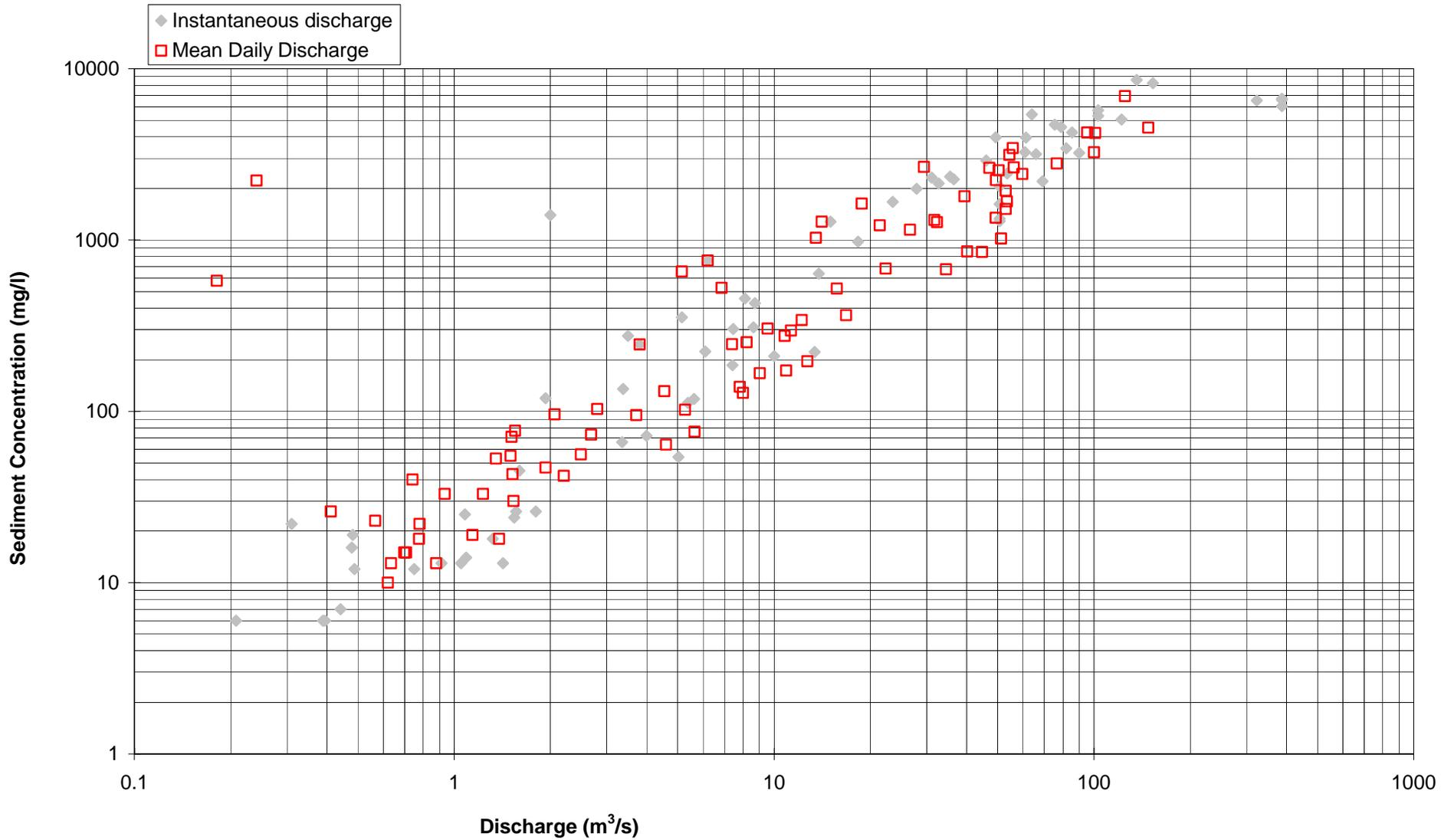
**Fig 5: Sediment Rating Curve for the Lesser Slave River at Highway 2A, 1977 - 1988.**
