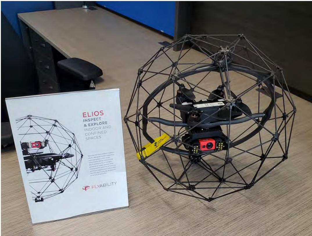
The “bucky ball” drone is designed for enclosed space inspections – the outer shell stops the propellers from striking objects. CUAV is advancing Beyond Visual Line of Sight (BVLS) operations, expanding the range remote pilots can reach from 1.5km to 11km. A great example of Calgary’s growing tech sector – thanks for the tour! Learn more at <https://canadianuavs.com/>
