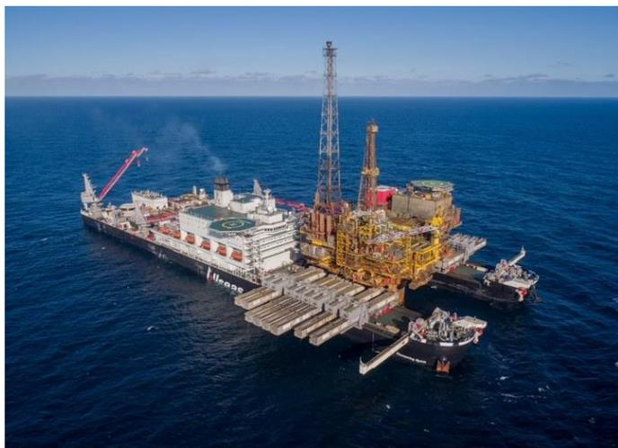
The DSME-built Pioneering Spirit has a width of 124 meters and can lift topsides of up to 48,000 tons in a single lift using eight sets of horizontal lifting beams.
