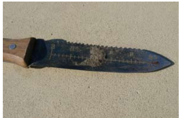
The hori hori weeding knife viewed from either side. One side is convex and tapered (above), the other concave and graduated (below).
