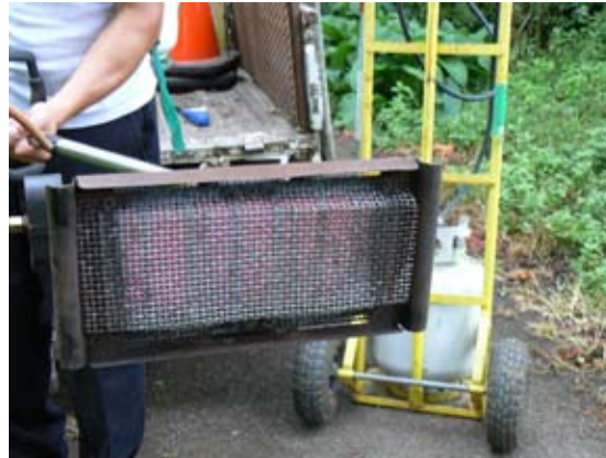
The Eco-Weeder (Puzzy Boy) model has a rectangular grill, with internal ceramic plates and is connected to a 20 pound propane tank sitting on a dolly.
