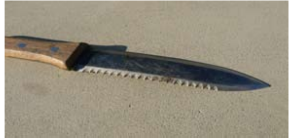
The hori hori weeding knife viewed from either side. One side is convex and tapered (above), the other concave and graduated (below).
