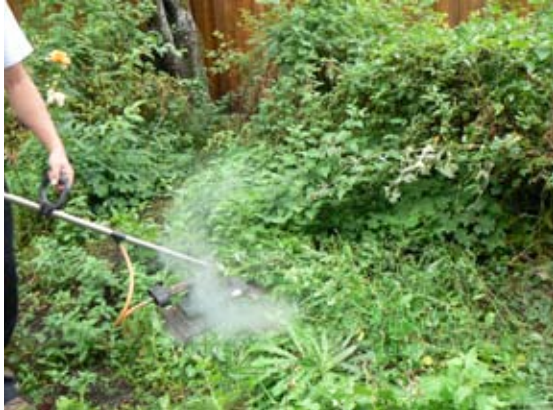
Steam rises from weeds seared by the Eco-Weeder (Puzzy Boy) in Scobert Gardens, a pesticide-free park in Eugene.
