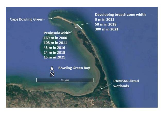
The peninsula width at the breach point is now only 15 m, compared to 24 m in 2018 and 108 m in 2011. The length of the breach zone is now about 300 m compared to 50 m in 2018.
