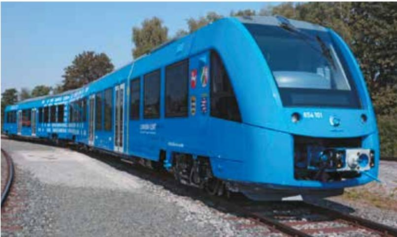
Lower Saxony is the pioneer regional Lander in Germany which is introducing a fleet of hydrogen trains to its regional rail network over the next few years<sup>22</sup>. 14 hydrogen trains will be in service by 2021 in Lower Saxony, which specified hydrogen trains as the preferred technology option for the network. Alstom's hydrogen train can reach 140 kmh, with a range of 600 to 800 km and accommodate up to 300 passengers
