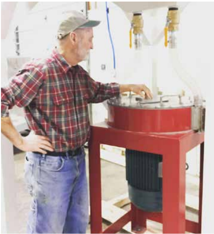
Darrold Glanville, co-founder of Sunrise Flour Mill, standing by the Unifine Mill, a high-velocity impact mill which shatters grain into tiny particles, creating a super-fine flour that retains the nutrition of the whole grain.
