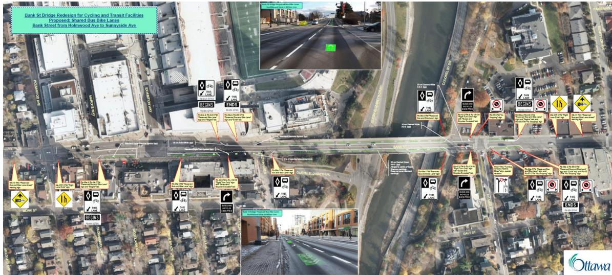
The lanes would be delineated with both Super Sharrows and diamonds painted on the road surface. In addition, there would be other pavement markings further demonstrating it was for the exclusive use of bicyclists and buses. In Figure C, a green stripe down the centre of the lane is shown as a possible lane marking. Staff would also consider hatched lines.
