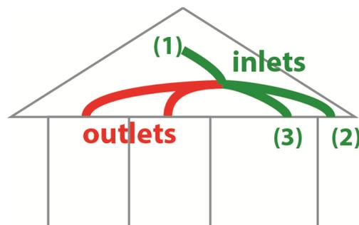
Systems with inlets from the roof cavity or outside are also known as "positive pressure" systems, as they draw in air from outside the home, which forces air out of other places (generally the same gaps that allow draughts in a home such as around door and window frames, through ceiling fans and vents, and between walls and floors, or walls and ceilings).
