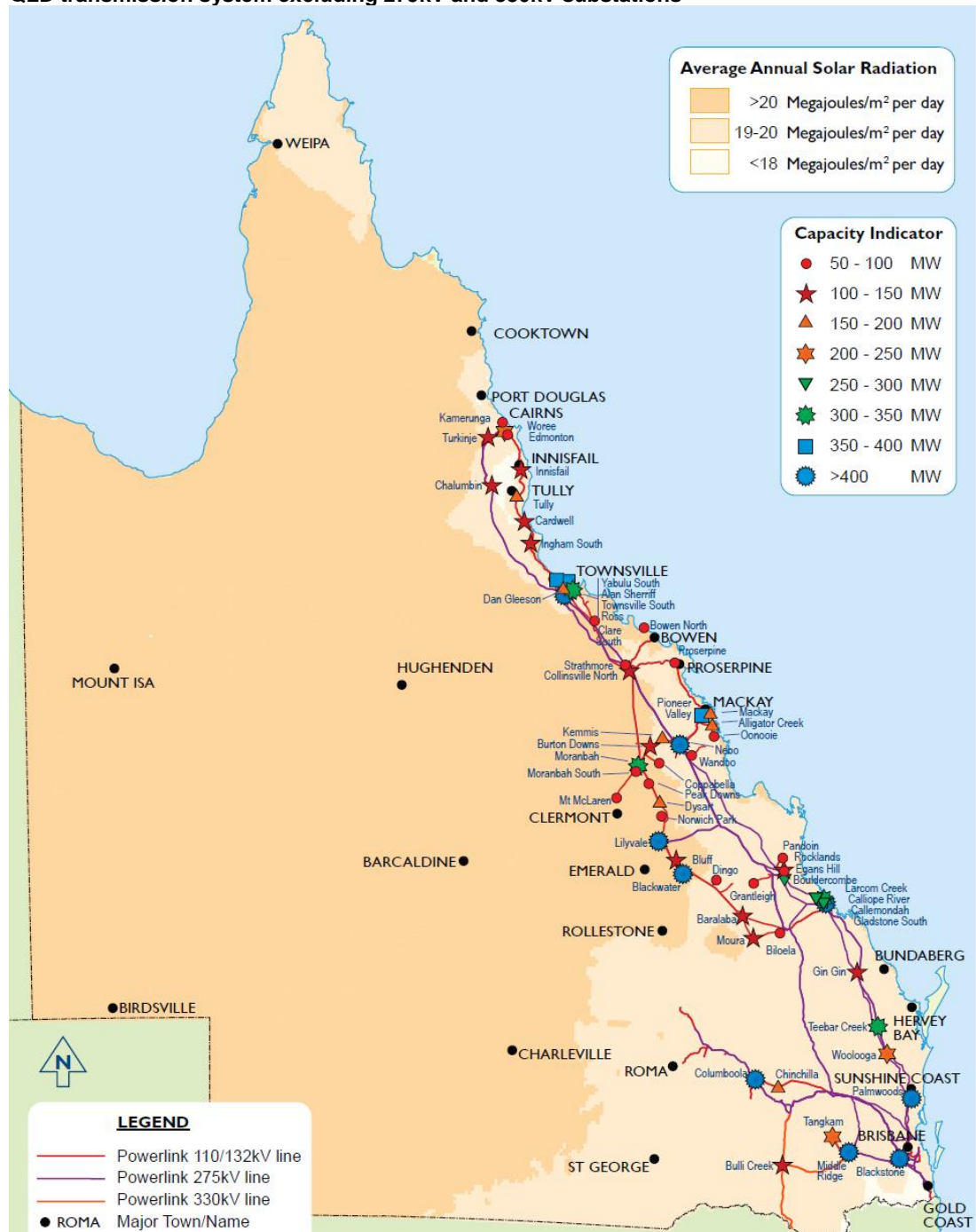
Figure 2-17 Powerlink assessment of the generation capacity that can be absorbed on the QLD transmission system excluding 275kV and 330kV substations
